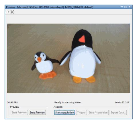
In the example shown here, the **Preview** panel of the Image Acquisition Tool is showing that frames are being acquired at an average of 30.93 FPS. The **Preview** panel also
